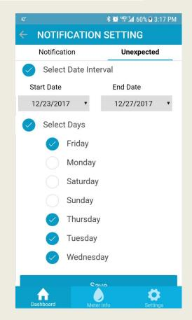
End-users can customize system to monitor for unexpected use. For example, if a homeowner is going on vacation they can program a begin/end date and provide an email alert if water is used while the homeowner's are away. Clauses are available for irrigation days to override the vacation start/end dates.
